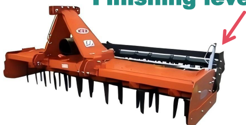
Finishing leveling roller
